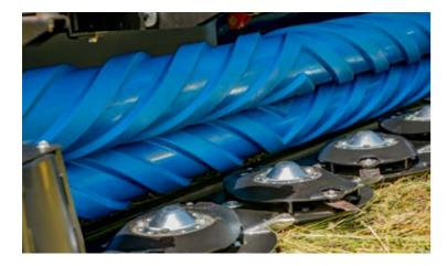
The **conditioning pressure is adjustable** by means of a lever control connected to torsion bars that adjust the roller spacing from 0 to 40 mm. In the latter position, the mown fodder passes between the rollers without being conditioned.
