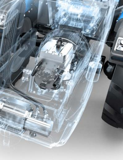
Under the bonnet of the e-Vanguard are two electric motors: the first 16 kW motor serves the hydraulic system, power steering and services while the second 25 kW motor is
